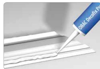
Apply the installation glue to the cornice
